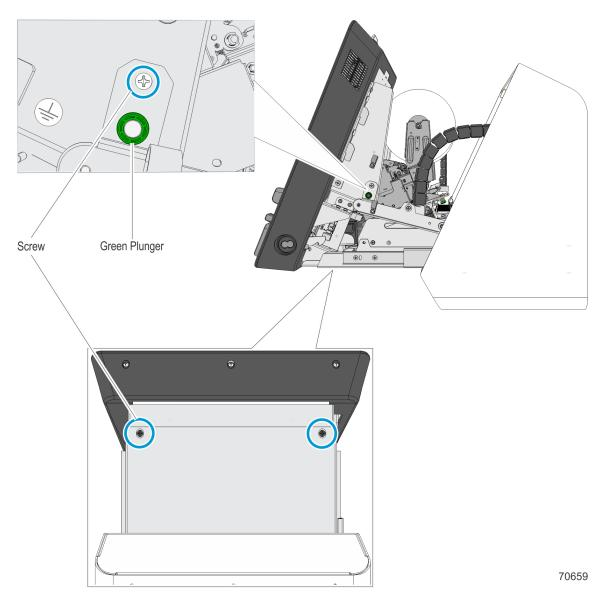
8. Pull the green plungers and twist it to a 90–degree angle on each linkage bracket, left and right, then lift the top of the unit forward until it stops.
