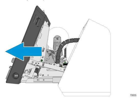
7. Remove the screw beside the green plunger on each side of the unit and the screws (2) at the bottom of the Display Head assembly.
