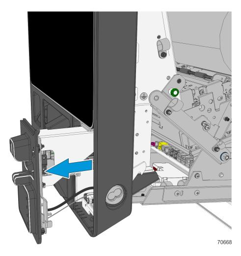
5. Unplug the NFC Modular Jack from the controller receptacle and the NFC Antenna Wire from the NFC module.
